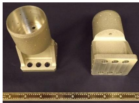
Figure 8: Additively manufactured spacecraft bracket. Courtesy of Ball Aerospace.
