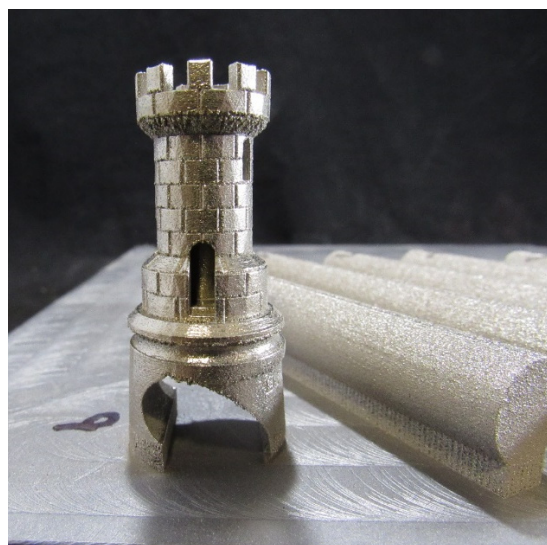
3D printed inconel superalloy test parts using René 80 as the base material.
