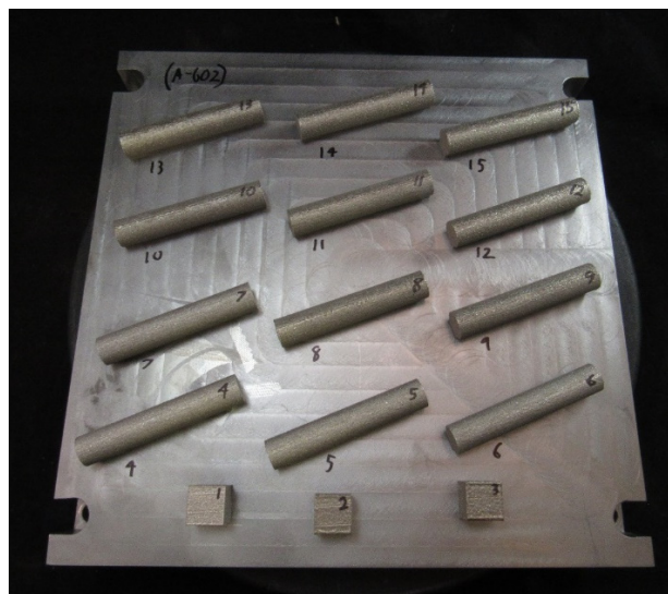
3D printed inconel superalloy test parts using 247 LC as the base material.
