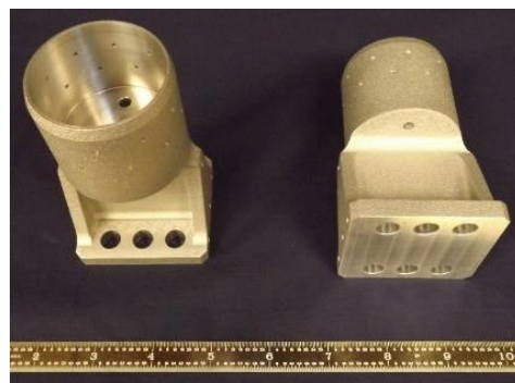
Figure 7: Additively manufactured spacecraft bracket. Courtesy of Ball Aerospace.
