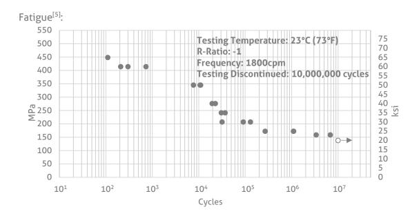
Properties stated on this data sheet are in the Elementum 3D prescribed HIP and T74 condition. <sup>[1]</sup>ASTM E8, <sup>[2]</sup>ASTM E18, <sup>[3]</sup>ASTM E494-20 (ultrasonic velocity), <sup>[4]</sup>Deposition rate calculation is for comparison purposes on an EOS M290 and does not include recoating time, laser migration time, contour exposures, etc. <sup>[5]</sup>ASTM E466, <sup>[6]</sup> Surface roughness determined by stylus profilometry.
