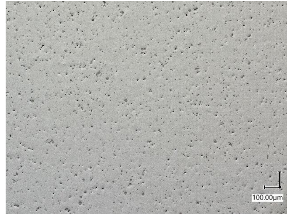
Figure 4: Image of A2024-RAM2 showing an even dispersion of ceramic particles and free of the microcracking seen in Figure 2 3. Taken at 100X magnification
